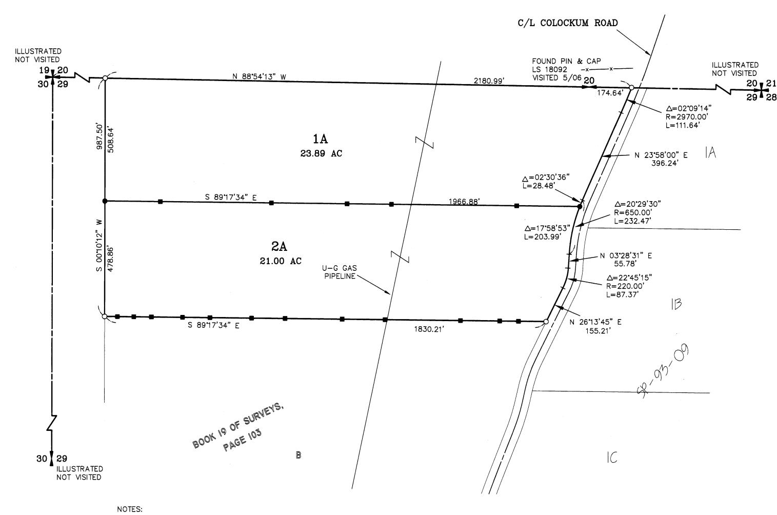
1. THIS SURVEY WAS PERFORMED USING A NIKON DTM 521 TOTAL STATION. THE CONTROLLING MONUMENTS AND PROPERTY CORNERS SHOWN HEREON WERE LOCATED, STAKED AND CHECKED FROM A CLOSED FIELD TRAVERSE IN EXCESS OF 1:10,000 LINEAR CLOSURE AFTER AZIMUTH ADJUSTMENT.
